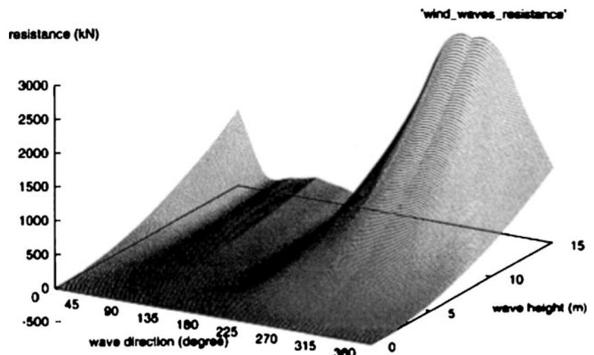
**Fig. 3** Example of added resistance to ship movement due to winds (Hoffschildt et al. 1999)
