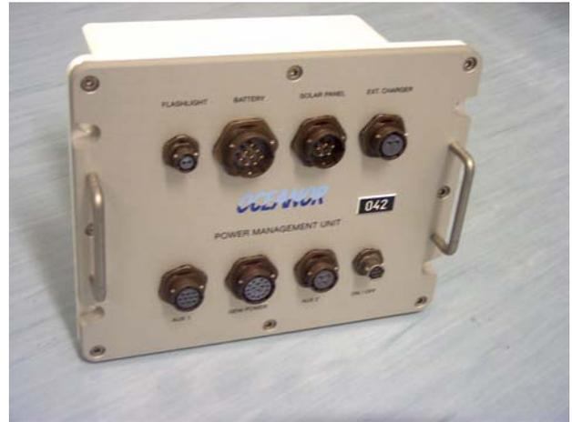
To provide fail-safe operation of the system, the Power Management Unit comprises two boards in a 2:1 redundancy configuration. One is configured as master (nominally active) and the other is configured as slave (nominally passive). An error situation detected in the master will raise a status flag, and the slave will automatically take over operation and inhibit the master.
