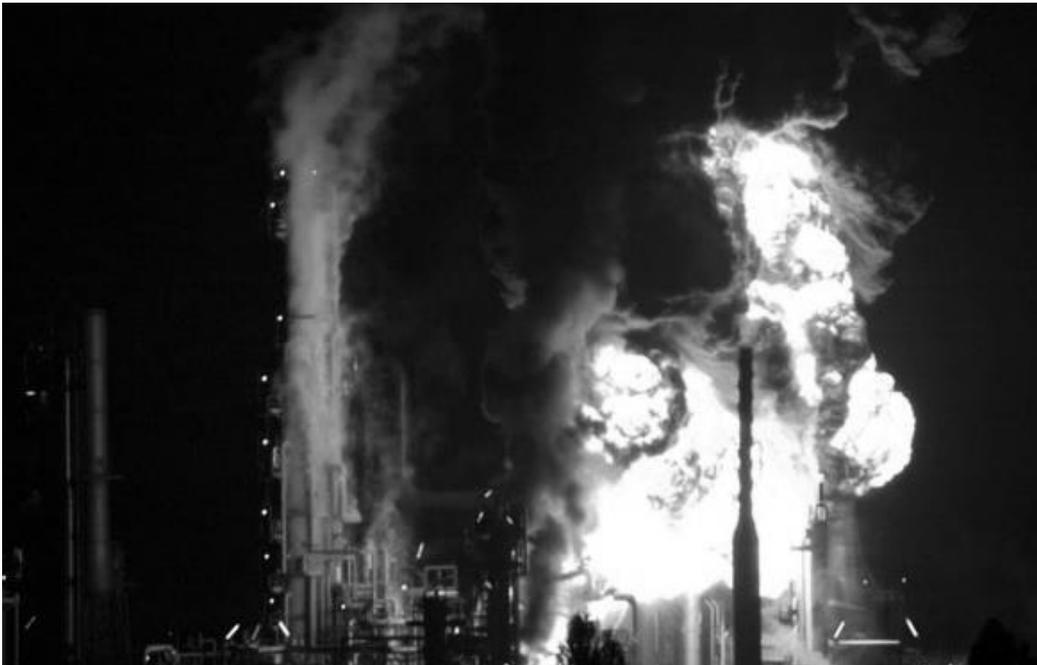
*Figure 2: Hydrogen jet fire originated at the Hydrodesulfurization reactor and following accident escalation with fire development of diesel oil in the nearby area.*
